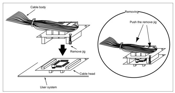
Figure 5 Fastening Cable Body
